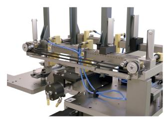
A changeover of Body Blank Length is done by the well known snap-in mechanism. A scale shows the current position. With the use of pre-set slot nuts a BBL changeover is done easily.
