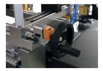
Depending on the sucker type and / or BBH dimension, a position correction of the support bars is necessary. Three predefined positions can be used, depending on body blank height, and may be adjusted by a snap-in mechanism.
