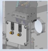
Manual setting of the gas flow rate with electric monitoring.
