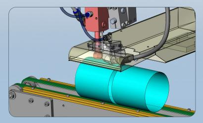
The container, filled with liquid lacquer, is put under pressure, which transports the liquid lacquer through the system to the spray gun. The sensor detects the can body as it approaches and transmits a control pulse to control valve, which activates the lacquer spray though spray gun **I**.
