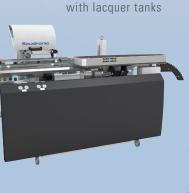
For cleaning and maintenance work in the outside seam application area, the lacquer drip pan can be removed without tools from its default position and placed in the stipulated service position above the conveyor belts. This protects the conveyor belts and drive mechanisms from any dirt and soiling created during maintenance work.
